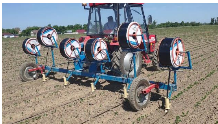
Figure 2. General view of the machine laying drip irrigation hoses between rows of cotton.
