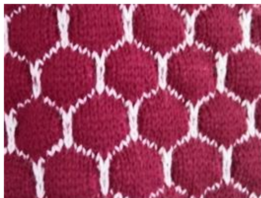
Figure 1. View and graph of two-layer knitted fabric Technological indicators of two-layer knitted fabric
