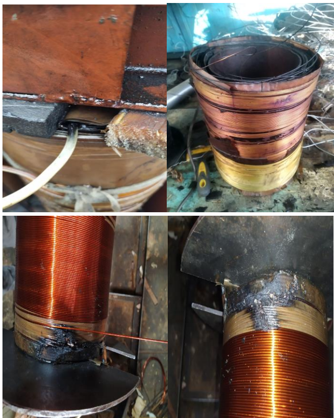
Figure 1. Burned and damaged cases of the transformer core.
