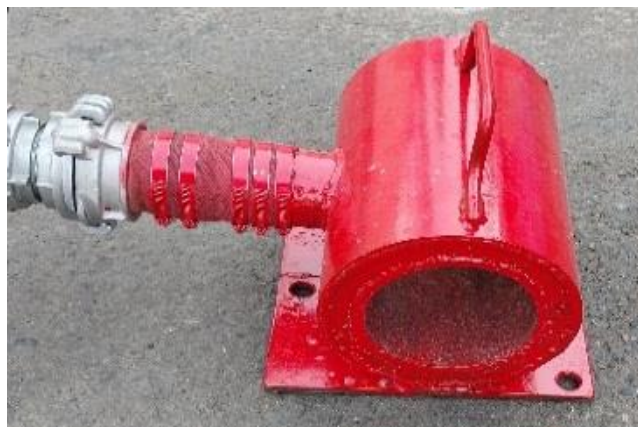
Rice. 2. General view of the device for intensive washing of fire hoses.
